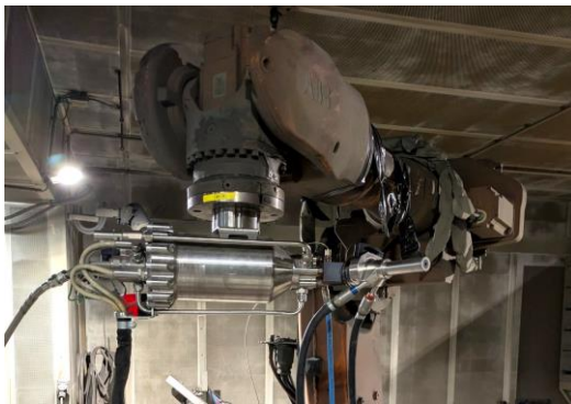
Robot-guided cold spray gun in the deposition cell
